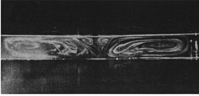
FIG. 2. Vertical structure of the model typhoons.
